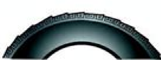
Diagonal Wear/ Heel and Toe Wear
